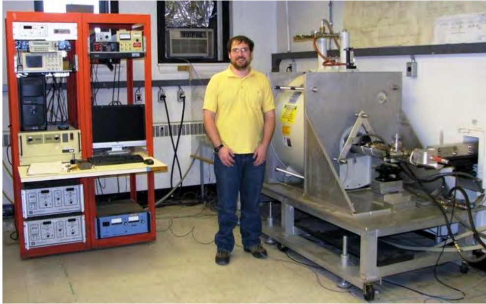
Fig. 2 A 140 GHz gyrotron oscillator used for DNP/NMR
