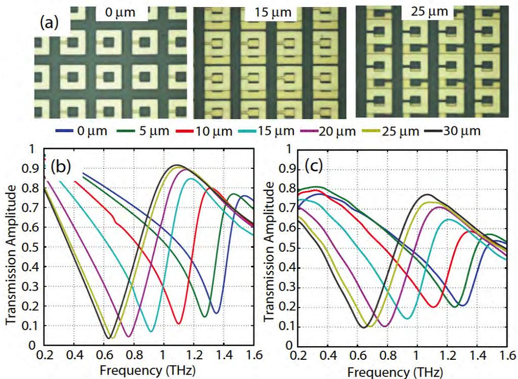
Fig. 3 (a) Optical micrographs of SRR structures shifted along the vertical direction for 0 (no shift), 15, and 25  $\mu\text{m}$ . (b) Simulation and (c) measurement results for THz transmission characteristics of the SRR structures shifted along the vertical direction for 0, 5, 10, 15, 20, 25, and 30  $\mu\text{m}$ . (Copyright to be applied)
