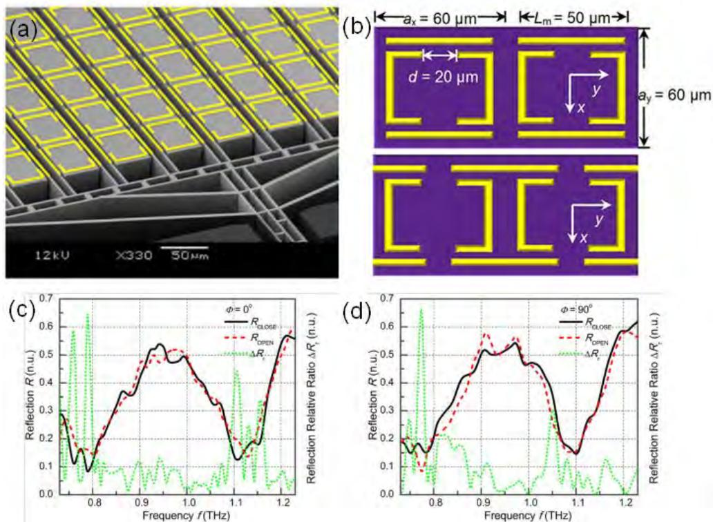
Fig. 2 (a) SEM images of the metamaterial structure in [112]. (b) Top schematic view of two elements in the CLOSE-state (top) and the OPEN-state (bottom). The reflection spectra under TE polarization in the CLOSE-state (dash) and the OPEN-state (solid) of the metamaterial when  $\Phi$  is (c)  $0^\circ$  and (d)  $90^\circ$ . Dotted line: the reflection relative ratio  $\Delta R_r$ . (Reprinted with permission from [112]. Copyright [2012], American Institute of Physics.)
