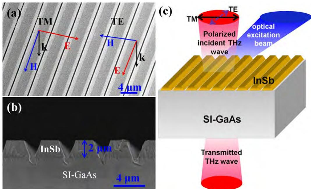
Fig. 8 (copyright to be applied) Scanning electron microscope (SEM) images of the fabricated InSb grating viewed from (a) top and (b) cross section. (c) Schematic of the transmission measurement configuration used in FTIR. The  $405\ \text{nm}$  *c.w.* laser is shone onto the InSb grating at an incident angle of  $\sim 45^\circ$ . Electric and magnetic field configurations of normally incident TE and TM waves are indicated in (a). H: magnetic field; E: electric field
