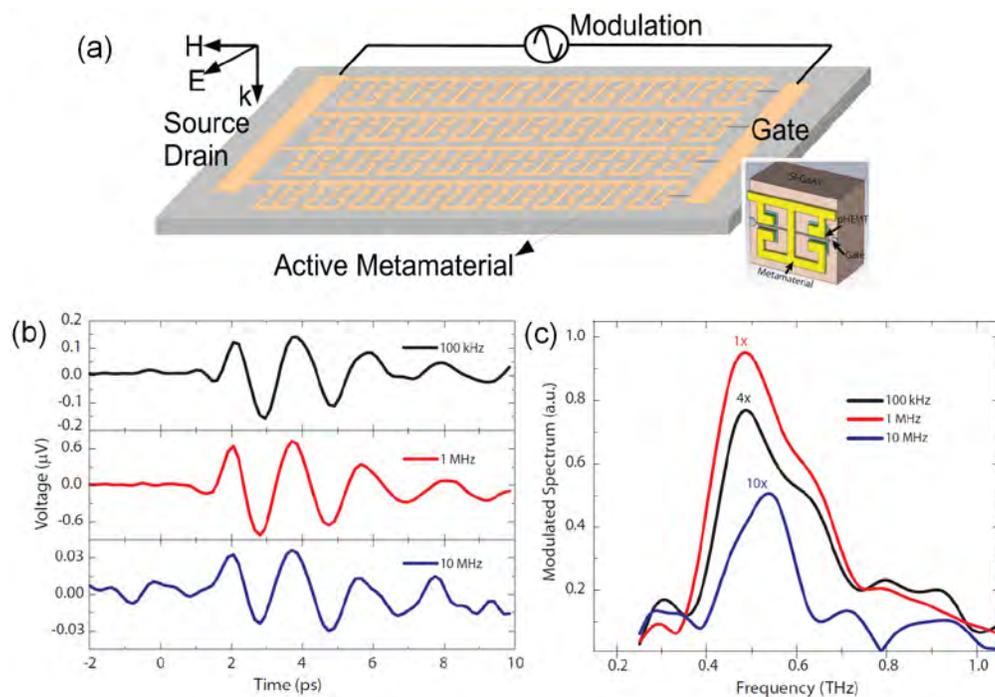
Fig. 7 (a) Active metamaterials hybrid Schottky diode, with inset showing the metamolecule. (b) and (c) show the THz time-domain signal and frequency spectra, respectively, at various modulation frequencies. (copyright to be applied)
