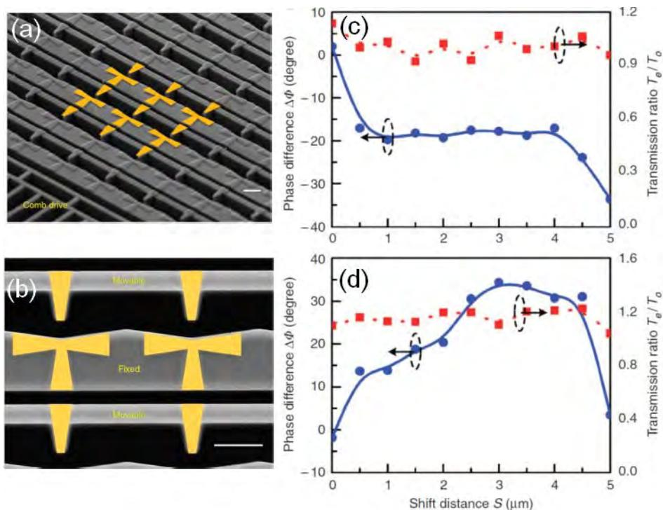
Fig. 5 anisotropic metamaterials based on Maltese-cross pattern (a) whole structure, (b) side view of metamolecules. The differential phase retardation and transmitted power ratio for (c) e- and (d) o-polarized light as functions of the shift distance. (Copyright needs to be applied by publisher)
