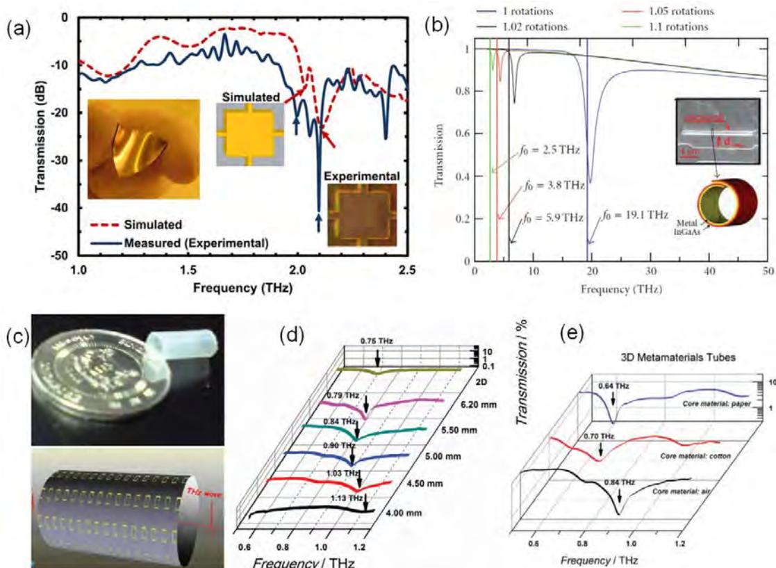
Fig. 12 (a) THz response of fishnet metamaterials on flexible PDMS substrate, inset: the device. Reprinted with permission from [140] Copyright [2012], American Institute of Physics. (b) Simulated responses of rolled-up THz metamaterials made of semiconductor materials, inset: the microroll. (copyright request submitted) (Copyright needs to be applied by publisher) (c) A 3D THz metamaterial tube, (d) and (e), tunable response with hollow and solid core, respectively.
