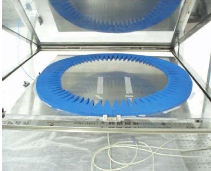
Fig. 4 The 2D near-field microwave scanning apparatus to measure the near fields shown in Fig. 2.
