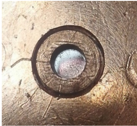
Fig. 2 The input window covered by the evaporated copper after electron bombardment
