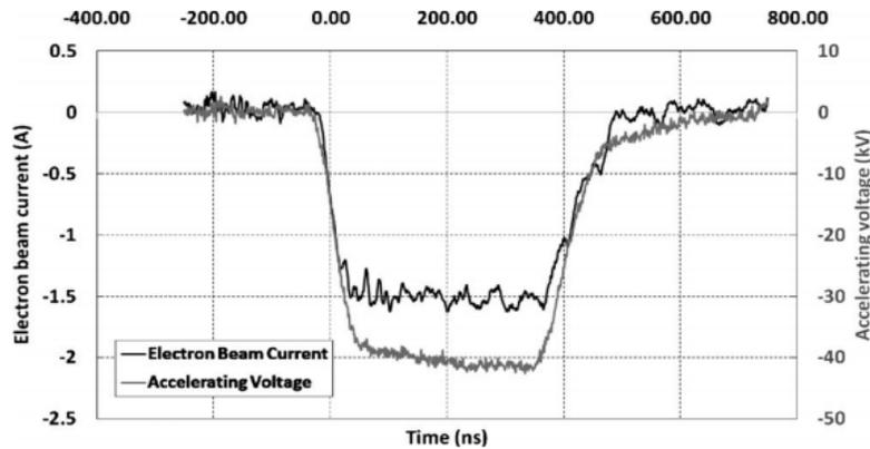
Fig. 6 The measured beam voltage and current.
