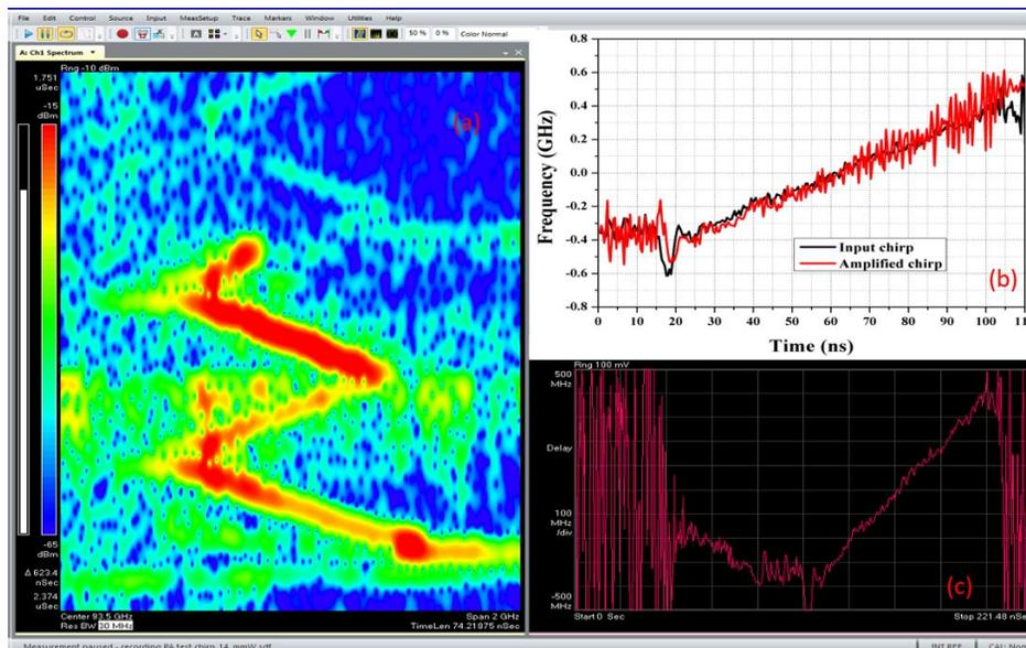
Fig. 16 Measurement of the frequency-swept amplification.
