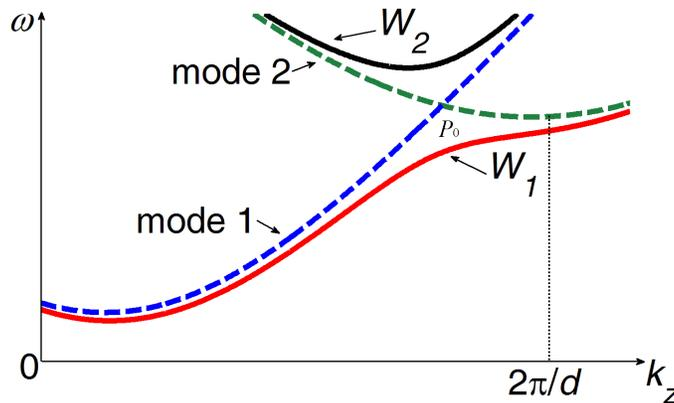
Fig. 3 The mode coupling in the HCIR
