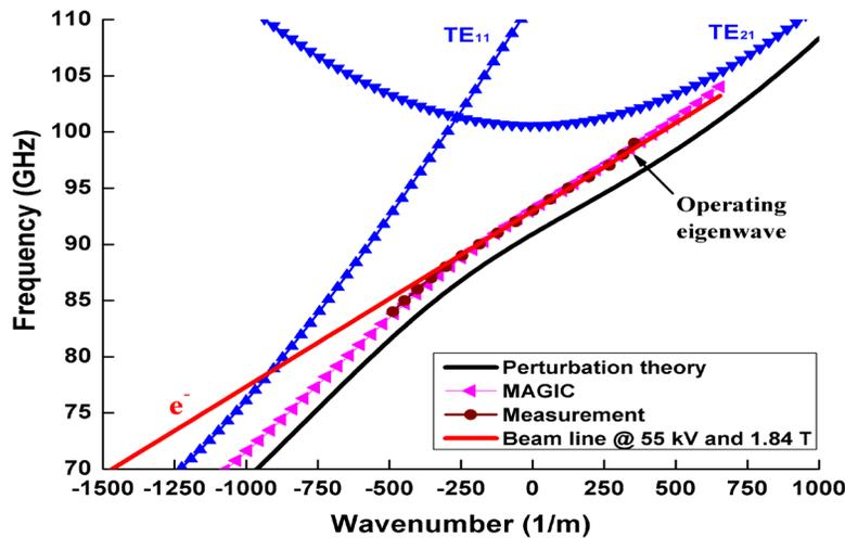
Fig. 4 The dispersion curve of the W-band gyro-TWA
