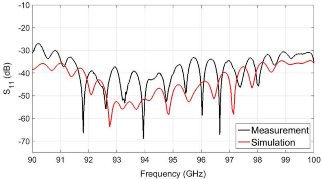
Fig. 13 The measurement of the multilayer microwave window.
