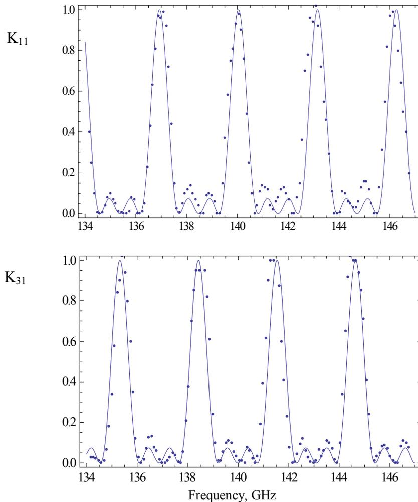
Fig. 5 The quadruplexer transmission functions for two outputs: solid curve – calculation, dots – experimental data.
