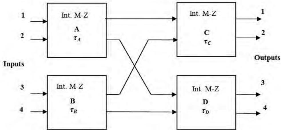
Fig. 2 The scheme of quadruplexer.
