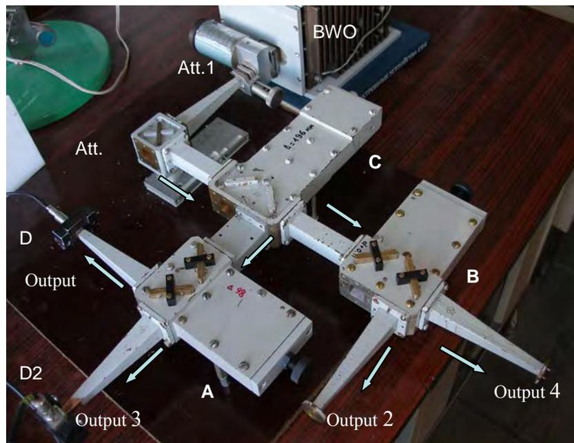
Fig. 3 The 140 GHz quadroplexer mock-up.
