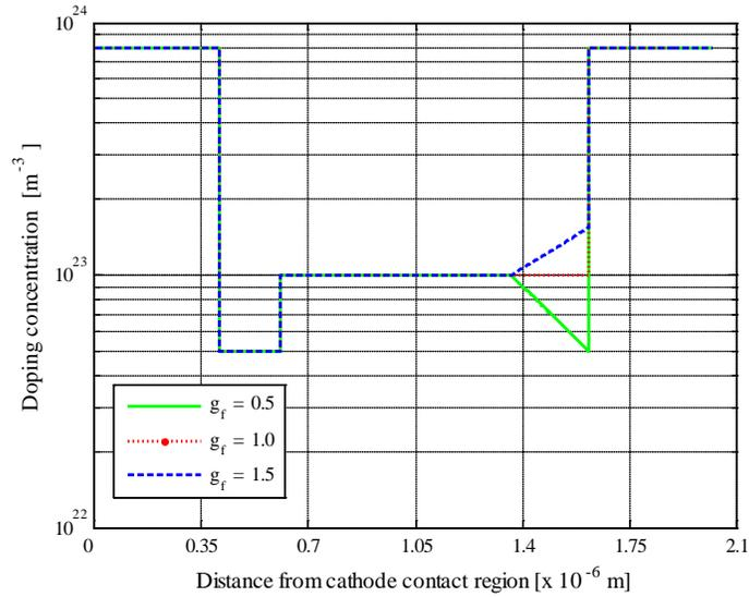
Fig. 1 Exponentially graded doping profiles of the benchmark, single domain  $0.175 \text{ THz}$  Gunn diode with doping notch at the cathode. The active region is sandwiched between two highly doped ohmic contact regions.
