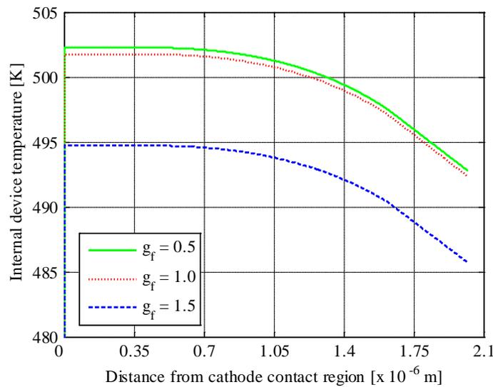
Fig. 3 Temperature profiles for different transit region doping concentration profiles with an ambient temperature of 300 K
