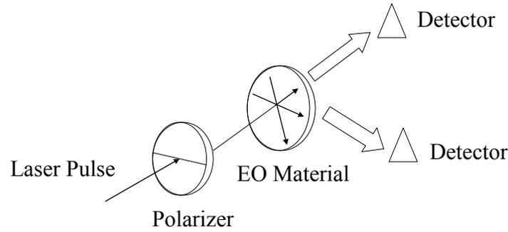
Fig. 2 The principle of the optical rectification effect for EO materials
