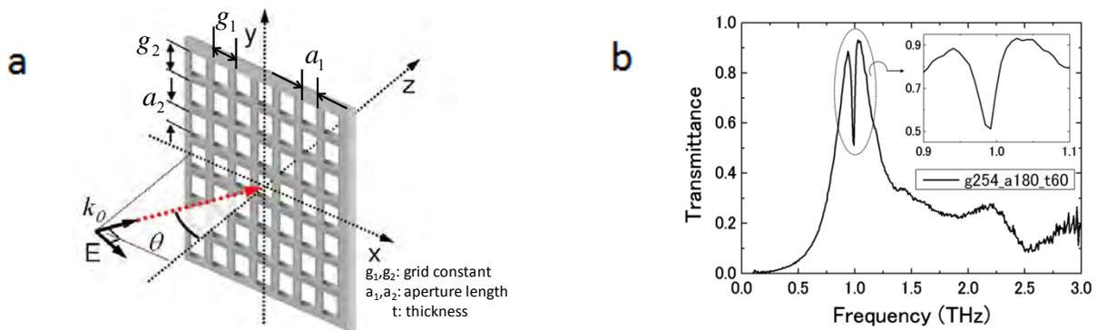
Fig. 1 Schematic and transmission spectrum of the metal mesh
