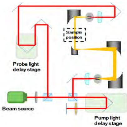
Fig. 2-1 Schematic of the THz-TDS system
