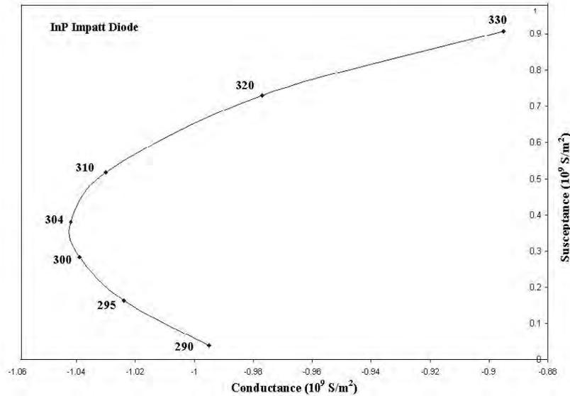
Fig. 4 Conductance-Susceptance plot of  $p^+ p-n^+$  double drift Indium Phosphide IMPATT diode at THz regime.
