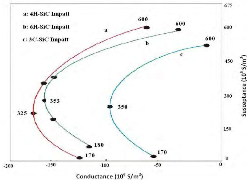
Fig. 2 Conductance-Susceptance plot of  $p^+pnn^+$  double drift Silicon Carbide IMPATT diodes at THz regime.
