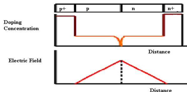
Fig.1 Schematic diagram of p+pn+ double drift Impatt diode and corresponding Doping and Electric Field profile.
