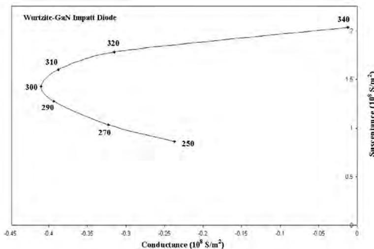
Fig. 3 Conductance-Susceptance plot of  $p^+pnn^+$  double drift Wz-GaN IMPATT diode at THz regime.
