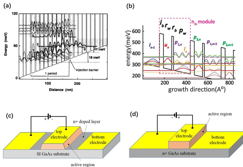
Fig. 1 Band structure of the active regions: (a) bound-to-continuum structure and (b) resonant phonon structure. Waveguide structure of (c) surface-plasmon waveguide and (d) metal-metal waveguide.
