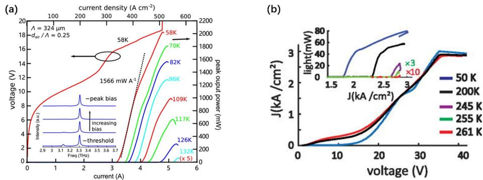
Fig. 3 Temperature dependent L-I-V curves for (a) the high-power single-mode device [41], (b) the high-temperature device [11].
