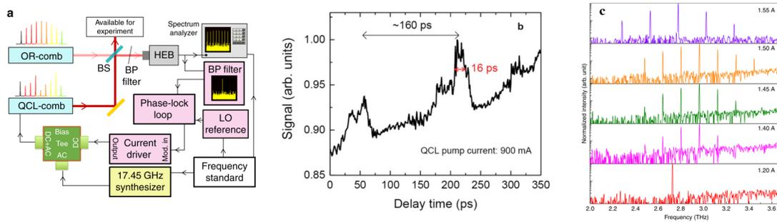
Fig. 4 (a) Schematics of the experimental setup employed for full stabilization of the THzQCL-comb based on dual-comb multi-heterodyne detection [46]. (b) Beam intensity of passively mode locked THzQCL-comb versus delay time [47]. (c) Spectra of THz frequency comb from mid-IR QCLs at room temperature continuous wave operation [48].
