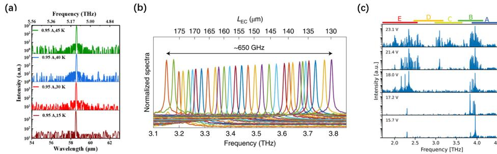
Fig. 2 Emission spectra of the THzQCLs. (a) The high frequency device [32], (b) the tunable single mode device[9], (c) the broad band device[10].
