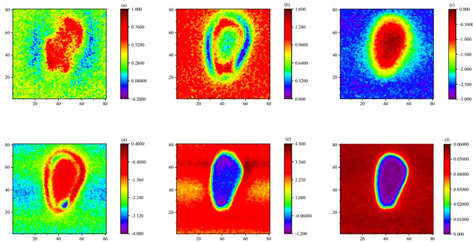
Fig. 4 Different image refactoring methods in Terapulse : (a)-14ps Time Slice; (b)-12ps Time Slice; (c)-10ps Time Slice; (d) Time Slice of  $-9ps-2ps$ ; (e) Time Slice of  $-13ps-11ps$ ; (f) Peak-peak Image.
