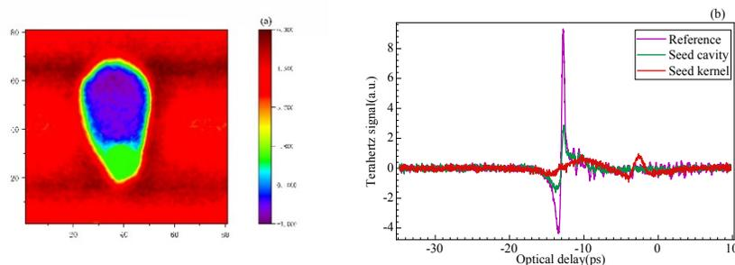
Fig. 3 Differential time slice and spectral comparison of samples : (a) Differential time slice of damaged sample; (b) Time-domain spectra at different locations
