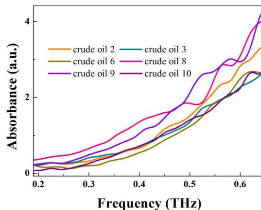
Fig. 3 THz absorbance spectra of tablets in a frequency range from 0.2 THz to 0.7 THz, respectively.
