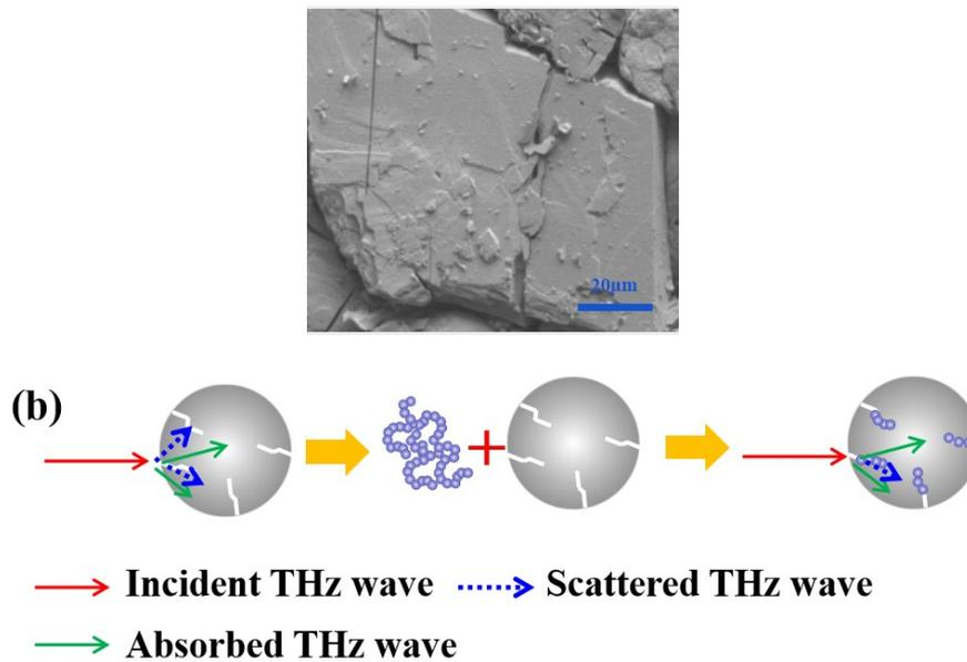
Fig. 6 (a) SEM image of quartz sand; (b) Schematic diagram of THz scattering.
