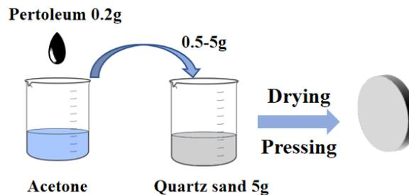
Fig. 1 The flow chart of sample preparation.
