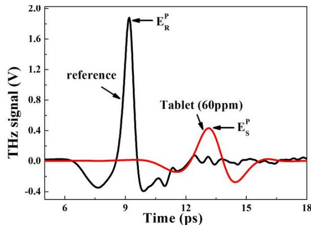
Fig. 2 THz-TDS of the reference and tablet with 60 ppm crude oil.
