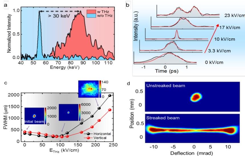
Fig. 5 Functions of the STEAM device. (a) Acceleration of electron beam with electron energy spectra for input beam (blue curve) and accelerated beam (red curve). (b) Temporal compression of the electron pulses as a function of the THz field in the rebunching mode. (c) Transverse electron beam focusing as a function of the THz field in the focusing mode. (d) Images of the electron beam on the detector with and without the THz deflection field in the streaking mode [6].
