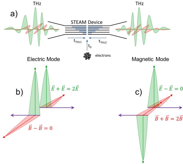
Fig. 3 a) Orientation of electric and magnetic fields relative to STEAM device b) Field orientations in the electric mode. c) Field orientations in the magnetic mode.
