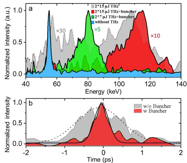
Fig. 7 Energy spread compensation. **a**, Measured electron energy spectra for input beam (Blue shaded curve), accelerated beam without buncher (gray shaded curve) and with buncher ( $2 \times 7$   $\mu$ J THz: green shaded curve and  $2 \times 15$   $\mu$ J THz: red shaded curve). The energy distribution is normalized to the 55 keV input electron beam with around 1 fC bunch charge. **b**, Measured input electron pulse duration with (red shaded curve) and without buncher (gray shaded curve). [9]
