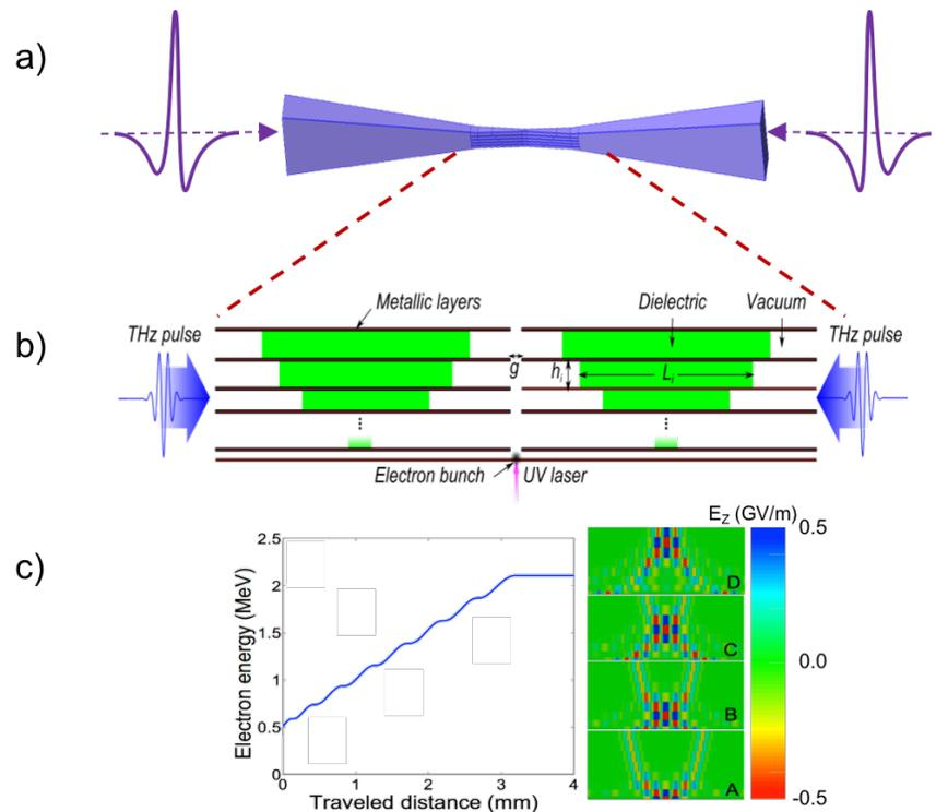
Fig. 2 a) Concept of segmented structure showing two input horns to concentrate the THz energy into the interaction region b) Diagram displaying the organization of the waveguide layers. c) Simulation showing acceleration of electrons from rest to  $2\text{ MeV}$  using  $2\text{ mJ}$  of THz energy [5, 8].
