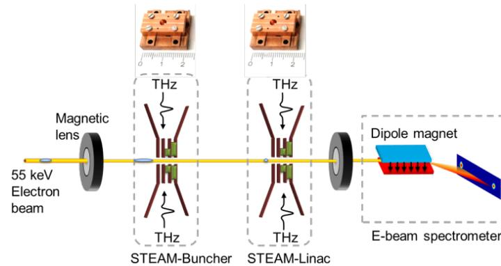
Fig. 6 Schematic illustration of the experimental setup. 55 keV electron bunches are generated by a DC electron gun. The STEAM-buncher is driven by two counter-propagating terahertz beams with energy  $\sim 2 \times 50$  nJ for electron compression. The STEAM-linac is driven by  $\sim 2 \times 15$   $\mu$ J THz radiation for electron acceleration. [9]
