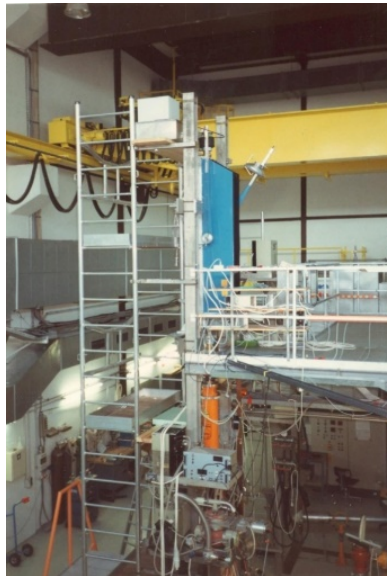
Fig. 5 Measurement of the mode purity of a TE_{10,4} -mode gyrotron using a wavenumber spectrometer.
