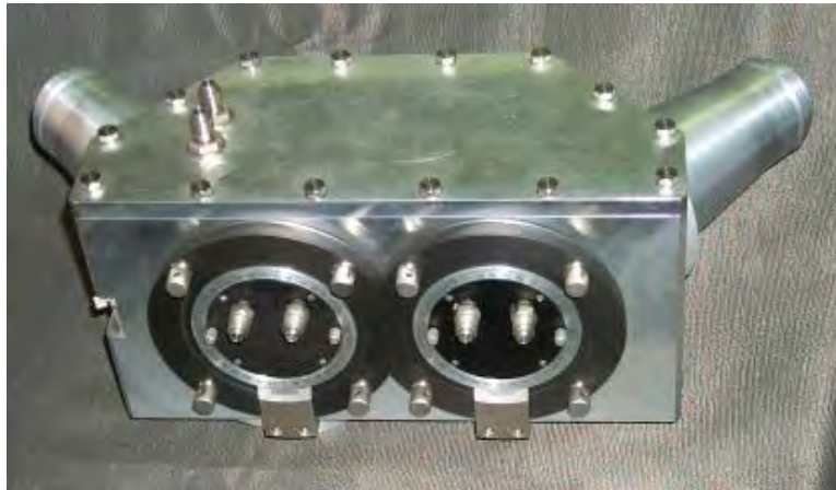
Fig. 4 An universal polarizer combined with a miter bend (courtesy by V. Belousov).
