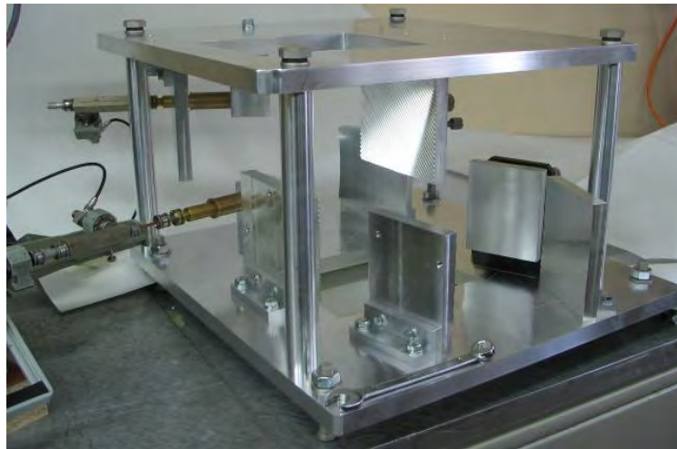
Fig. 6 W-band duplexer (transmit-receive isolation -45 dB, bandwidth 8%).
