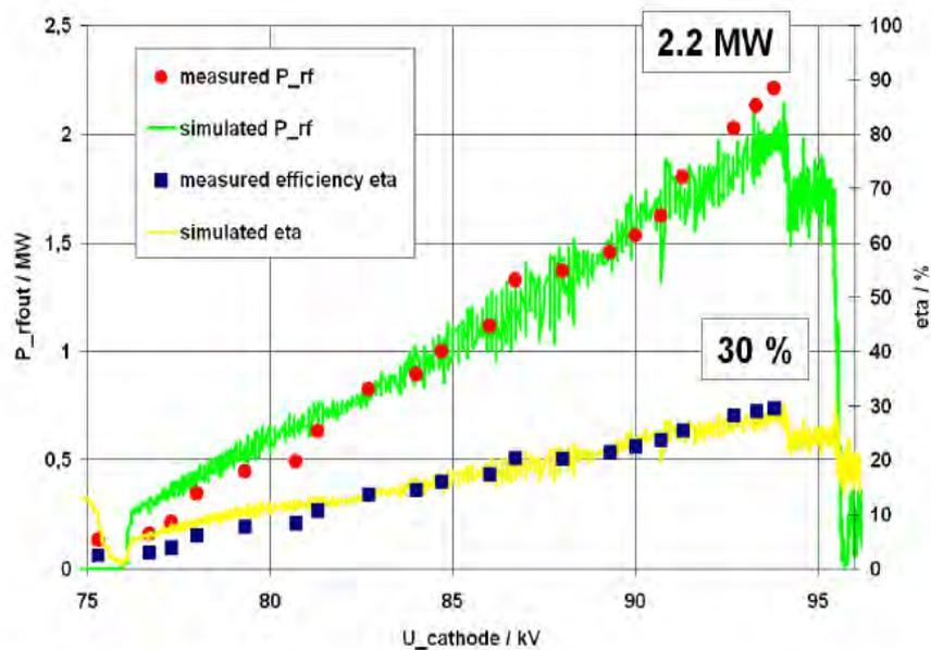
Fig. 6 Measured and calculated gyrotron output power and efficiency vs. cathode voltage at the nominal magnetic field of 6.87 T.
