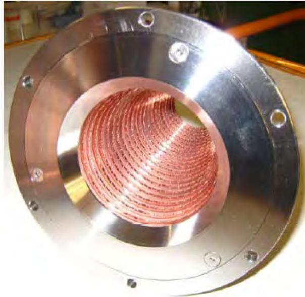
Fig. 5 Photo of the new beam tunnel with irregularly longitudinally corrugated copper rings.
