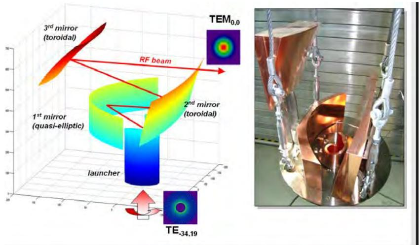
Fig. 8 Quasi-optical mm-wave output coupler of the coaxial-cavity gyrotron.
