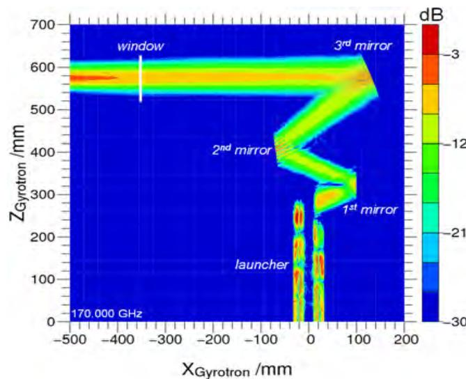
Fig. 9 Millimeter-wave beam propagation in the improved q.o. output coupler calculated with the SURF3D code [15].
