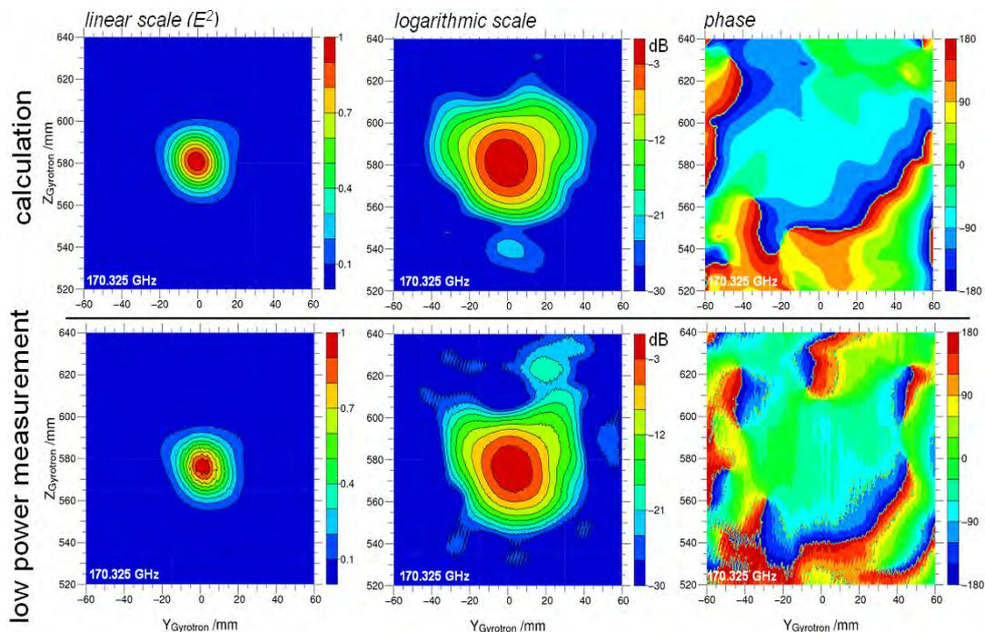
Fig. 11 Calculation (upper) and low power measurement (lower) of the mm-wave beam profile and phase distribution at a distance of 500 mm outside the gyrotron window.
