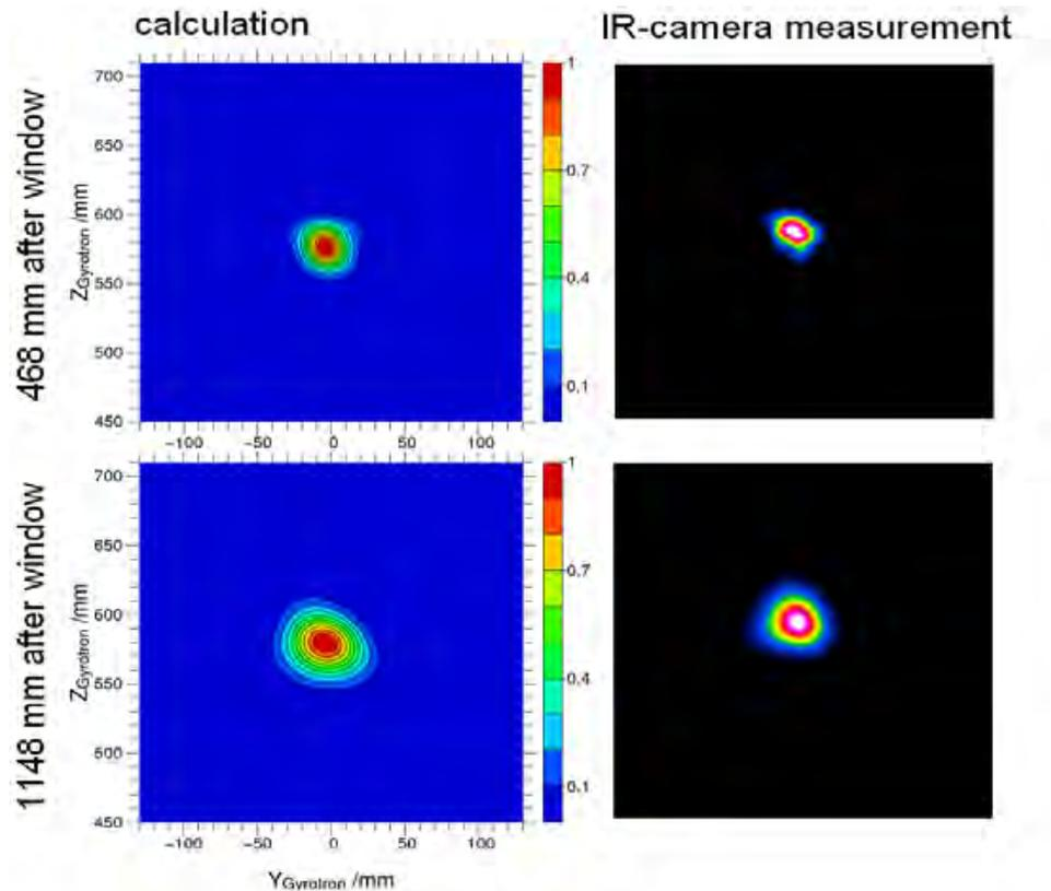
Fig.13 Calculations (left) and high-power IR-camera measurements (right, with the same scales) of the mm-wave beam profile for the gyrotron operation at  $0.1433 \text{ THz}$  in the  $\text{TE}_{29,16}$  mode.
