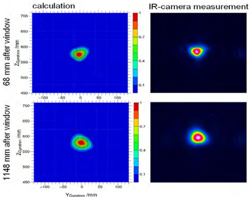
Fig.12 Calculations (left) and high-power IR-camera measurements (right, with the same scales) of the mm-wave beam profile for the gyrotron operation at 0.17 THz in the TE<sub>34,19</sub> mode.
