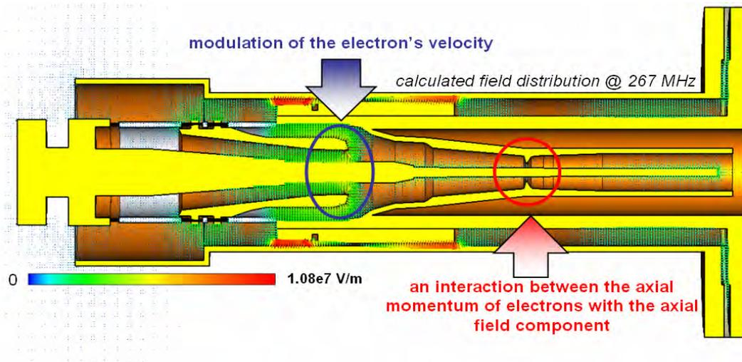
Fig. 3 Calculated field distribution at 267 MHz – regions responsible for the excitation of the parasitic oscillation are indicated.
