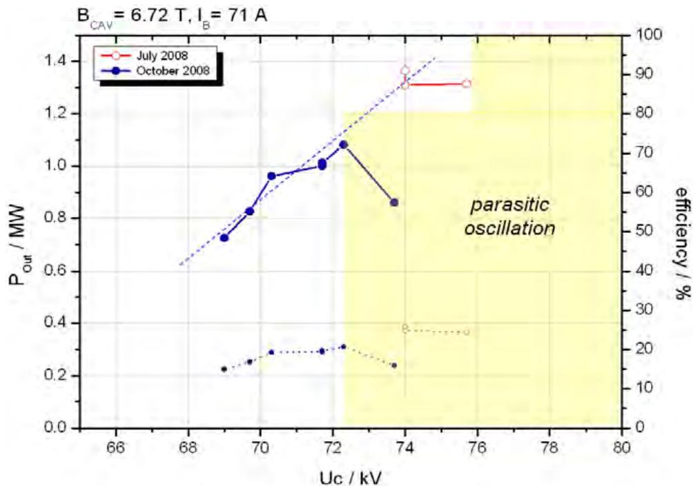
Fig. 4 Measured gyrotron output power and efficiency vs. cathode voltage at reduced cavity magnetic field. Destructive influence of parasitic oscillations around  $0.16\text{ THz}$  to  $0.17\text{ THz}$  on the power generation in the coaxial cavity has been observed during the experiment.
