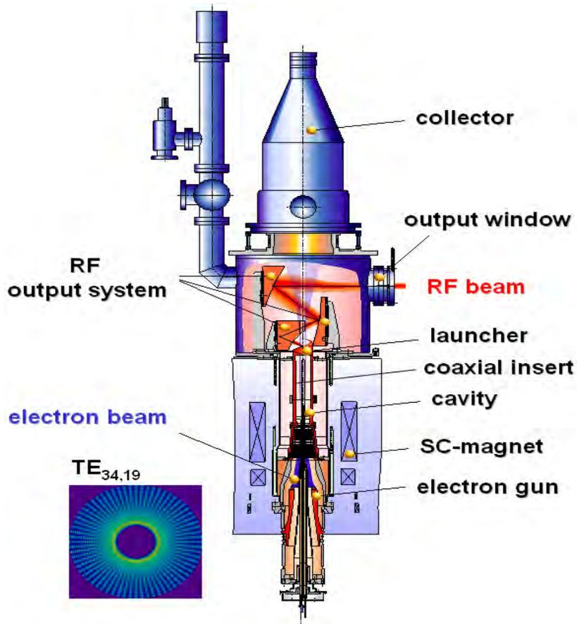
Fig. 1 Short-pulse 0.17 THz, 2 MW coaxial-cavity gyrotron at KIT (pre-prototype tube).
