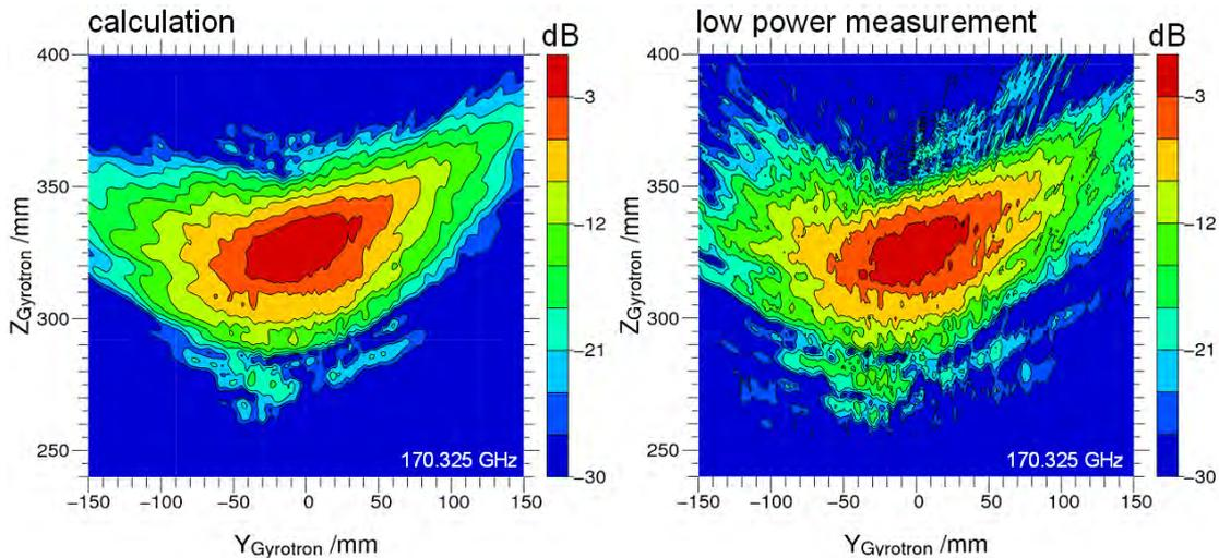
Fig. 10 Radiated field of the new launcher in a plane at a distance of 100 mm from the launcher axis, calculated using the SURF3D code (left) and measured at low power (right).
