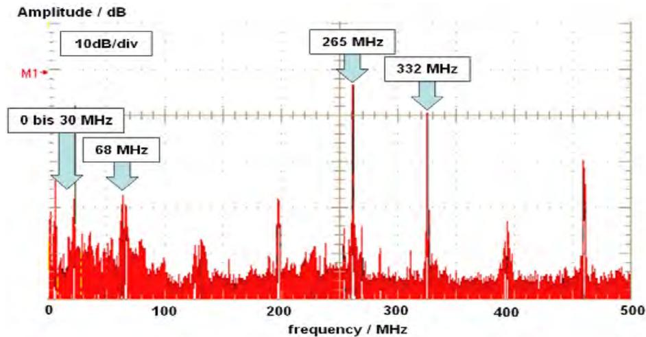
Fig. 2 Measured spectrum of the parasitic low frequency (LF) oscillations.
