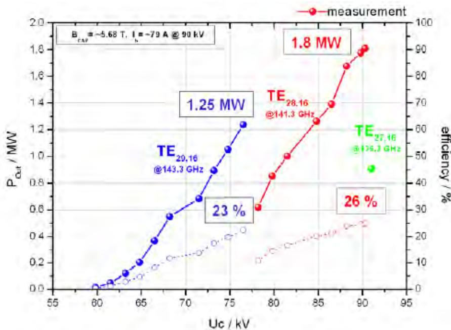
Fig. 7 Measured output powers and efficiencies vs. cathode voltage during frequency-step tunable operation in the TE<sub>28,16</sub> mode at 0.1413 THz and the TE<sub>29,16</sub> mode at 0.1433 THz.
