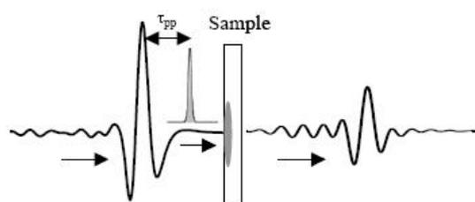
**Figure 1.** Schematic illustration of the effect of photoexcitation on the transmitted THz pulse. The entire waveform can be analyzed to obtain the frequency dependent complex conductivity, or the maximum point on the THz waveform can be recorded as a function of pump-probe delay time to measure the average conductivity as a function of time, and this is known as a THz “pump scan”.
