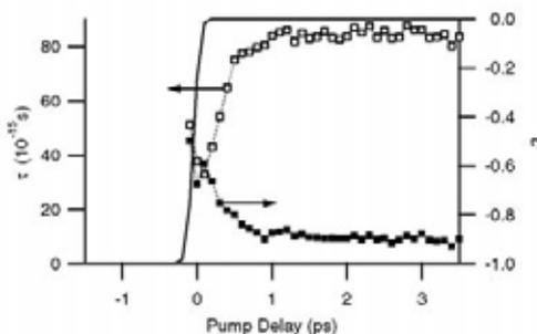
**Figure 4.** Plot of the carrier scattering time  $\tau$  (open squares) and  $c$  (solid squares) as a function of pump delay time based on global fit described in Ref. 10. The solid line indicates the onset of photoconductivity.
