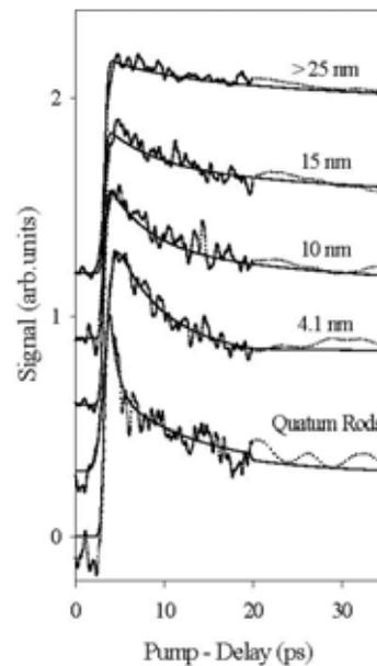
Figure 6. 1D pump delay scans of CdSe quantum dots of various sizes. Smooth curves are triple-exponential fits.
