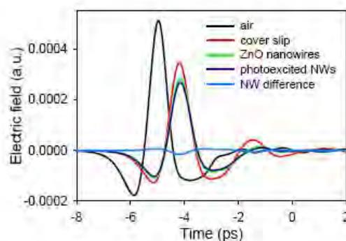
**Figure 2.** The black line is the THz pulse with no sample in the beam path. The red line shows the effect of the glass cover slip on the THz pulse. The green line is that of the ZnO nanowires on top of the glass cover slip. The dark blue line shows the THz transmission after photoexcitation of the ZnO sample. The light blue line is the THz “difference scan” when a chopper is placed in the excitation laser beam path, and a lockin amplifier is used.
