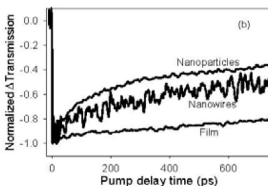
**Figure 5.** Decrease in photoconductivity as a function of pump-probe delay time for various ZnO morphologies.
