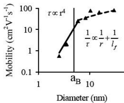
Figure 7. Mobility in CdSe NPs as a function of size.
