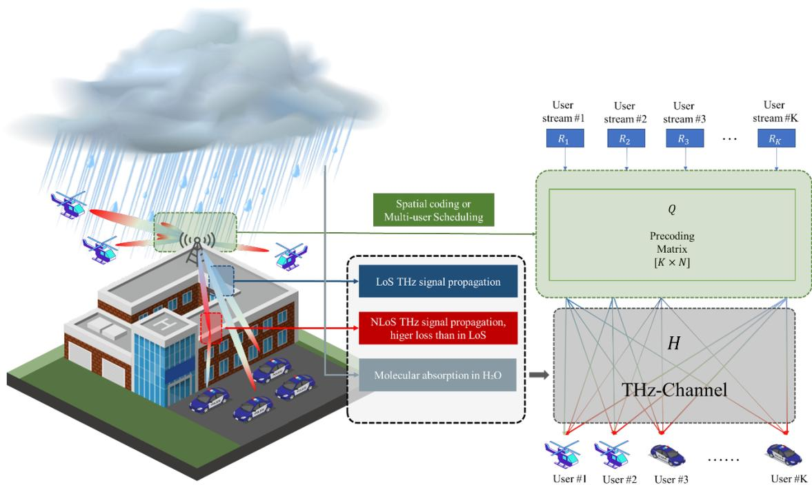
Fig. 3 Mitigating water molecule absorption and path loss in rainy weather at a police station scenario by using massive MIMO.
