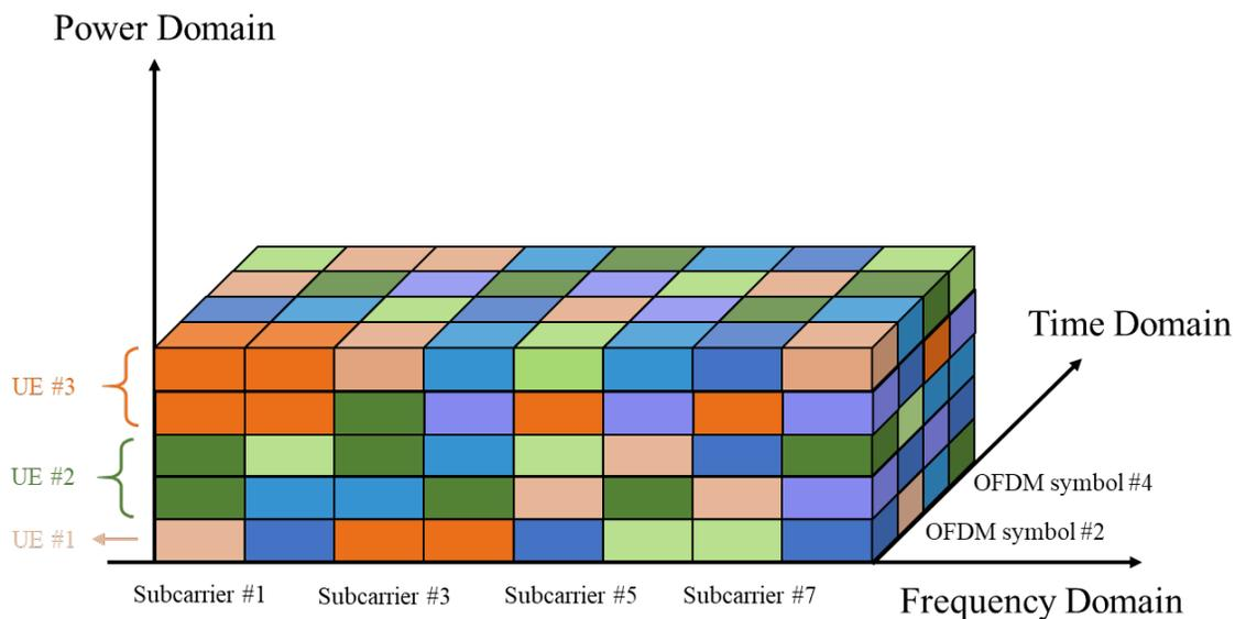
Fig. 2 Resource mapping in time, frequency and power domain using NOMA, same RB at the first subcarrier and the first OFDM symbol is used within different users, distinguished by power (value denoted by color).
