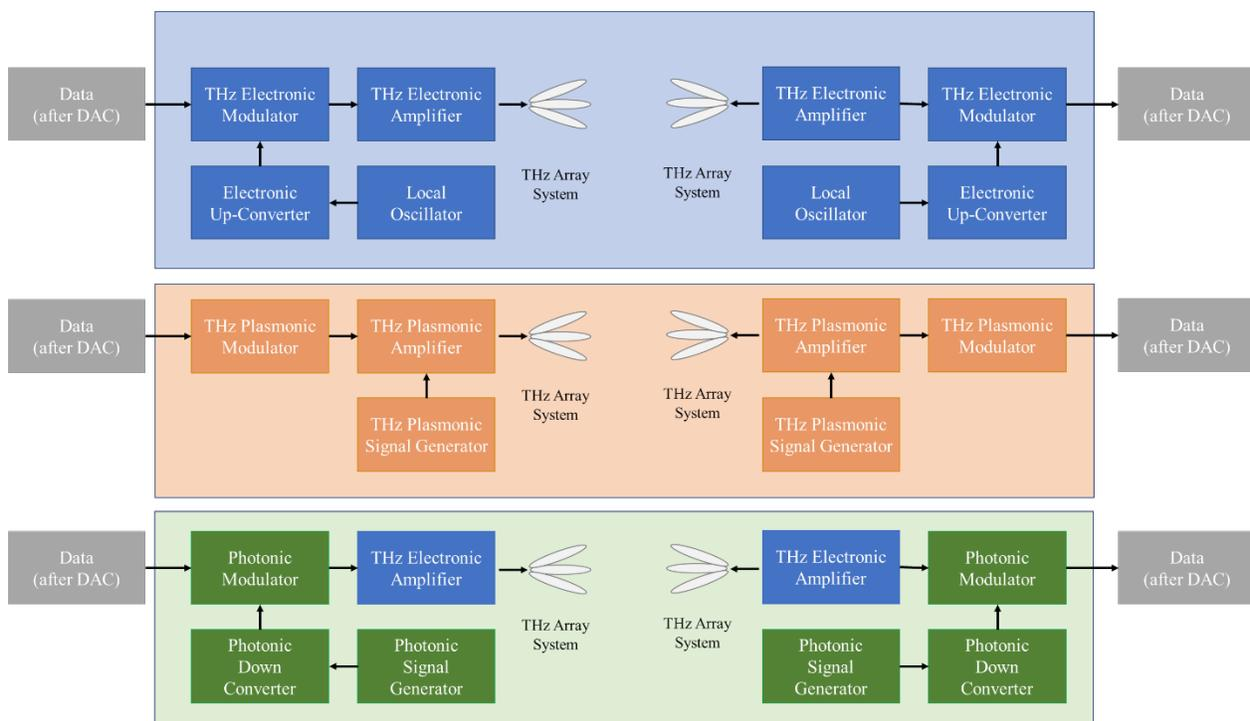
Fig. 5 Main components of different types of THz transceivers.
