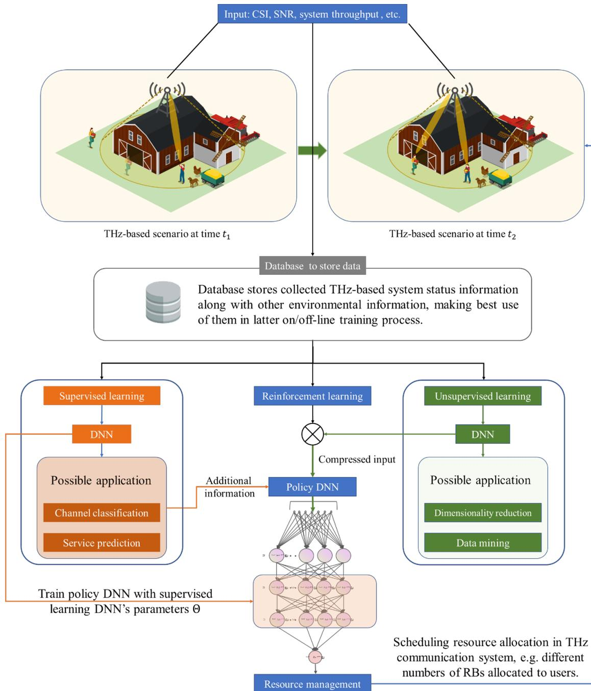
Fig. 7 An autonomous ML-based THz resource management system making full use of collected THz system status.
