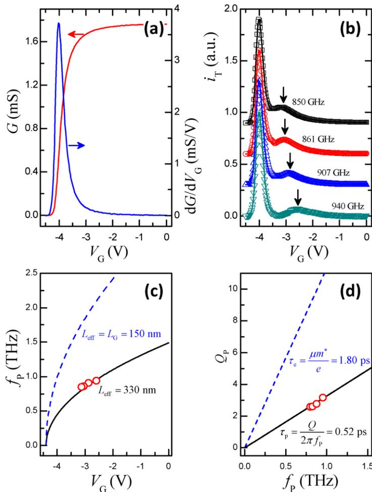
Fig. 6 Resonant and non-resonant plasmon detection in the antenna-coupled field-effect transistor. (a) The channel conductance as a function of the gate voltage  $V_{G1}$ . (b) The photocurrent as a function of the gate voltage  $V_{G1}$  at different terahertz frequencies. (c) Extracted resonant frequency as a function of the gate voltage. (d) Extracted quality factor of plasmon modes. The device is cooled down to 77 K.
