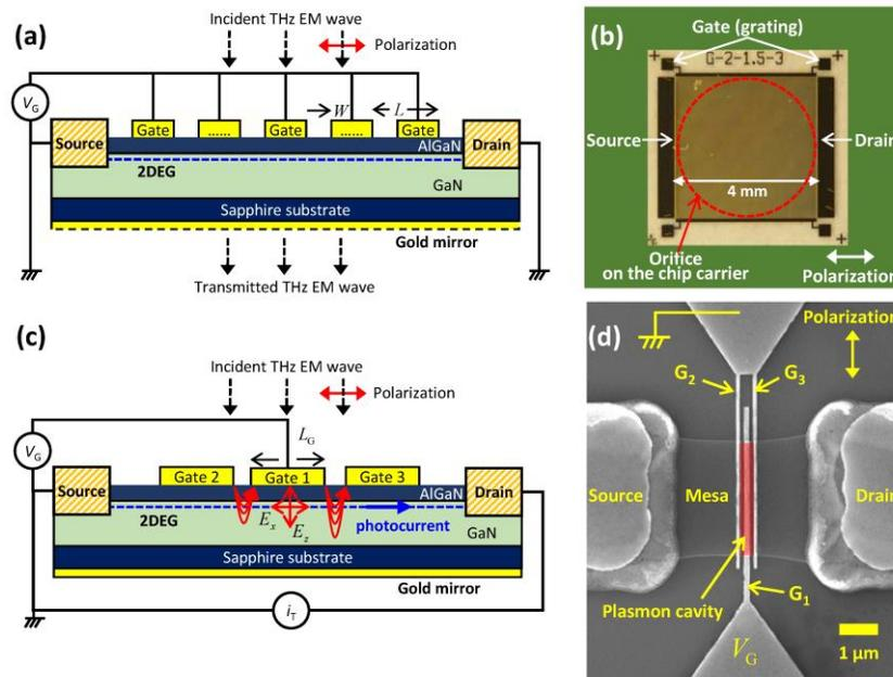
Fig. 2 (a) Schematic and (b) micrograph of the grating-coupled field-effect transistor. (c) Schematic and (d) micrograph of the antenna-coupled field-effect transistor.
