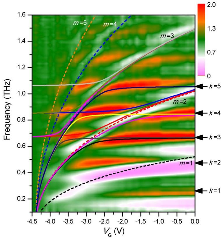
Fig. 4 Transmission spectra at different gate voltages obtained from the grating-coupled field-effect transistor cooled down to 8 K. The spectra were measured using a terahertz time-domain spectrometer (THz-TDS). Refer to Ref. 18 for the same measurement setup. Similar transmission spectra (worse signal-to-noise ratio comparing to the THz-TDS data) were obtained by using setup shown in Fig. 3.
