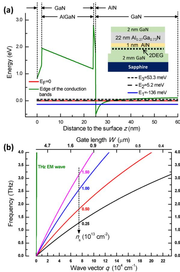
Fig. 1 (a) Conduction-band diagram of an AlGaN/GaN heterostructure from a self-consistent calculation. The 2DEG is formed in the GaN quantum well where
