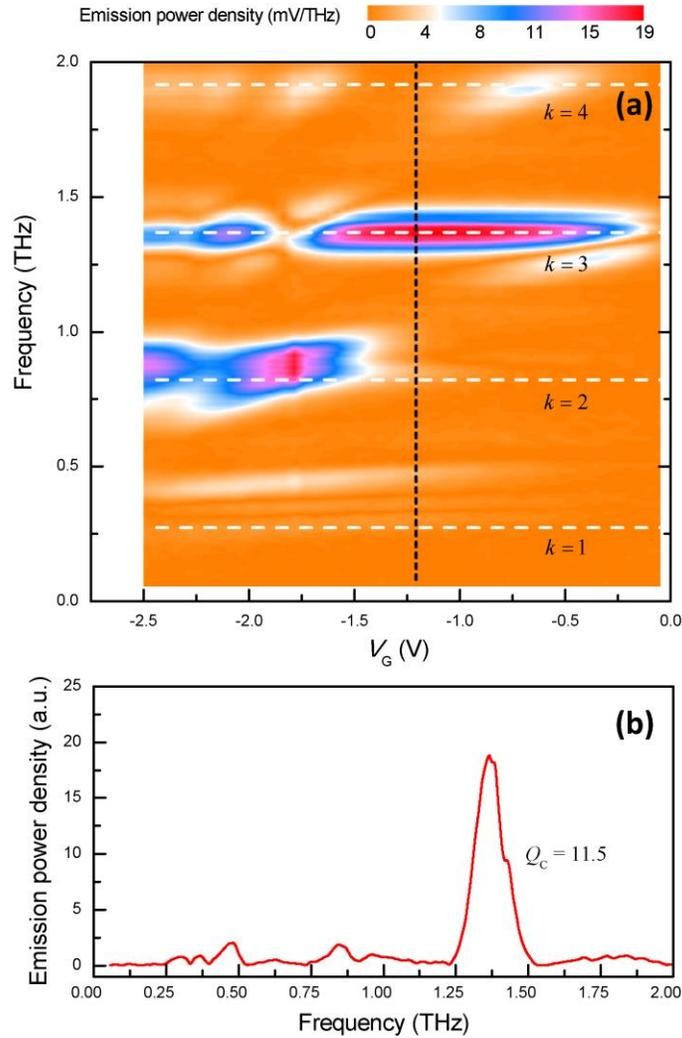
Fig. 5 (a) Emission spectra at different gate voltages. (b) A single emission spectrum at  $V_G = -1.22$  V. Obtained from a grating-coupled field-effect transistor with the sapphire substrate thinned down to  $91 \mu\text{m}$ . The device was cooled down to 8 K.
