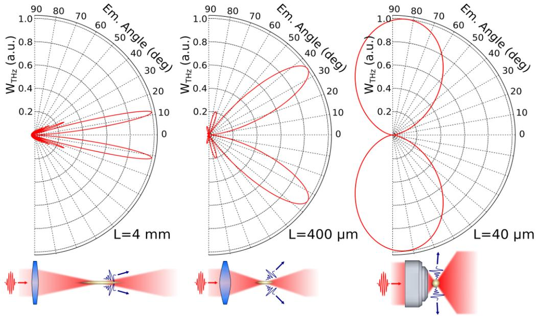
Fig. 5 Computation of THz pulse energy as a function of emission angle for three different values of plasma lengths. From left to right, the plasma length is 4 mm, 400  $\mu\text{m}$ , and 40  $\mu\text{m}$  respectively.
