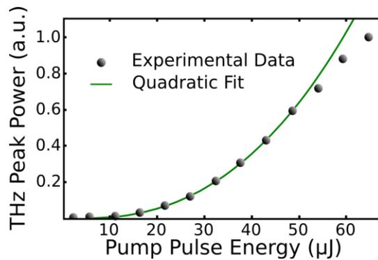
Fig. 4 THz pulse peak power vs. pump pulse energy. The detection angle was 80 degrees. The solid dots correspond to the experimental data, while the solid line is the best quadratic fit.
