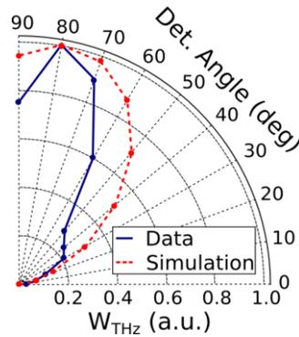
Fig. 6 THz pulse energy as a function of detection angle. The pulse energy is computed from the THz waveforms displayed in Fig. 2(a). The solid line is the experimental data, while the dashed line is the simulation obtained with the model described in [23].
