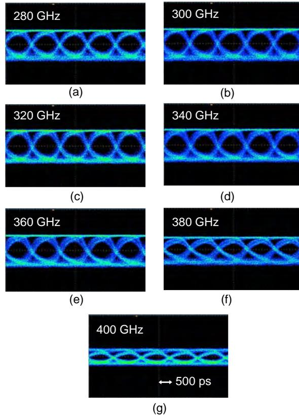
Fig. 14 Eye diagrams at a bit rate of 1 Gbit/s with carrier frequencies from 280 GHz to 400 GHz.
