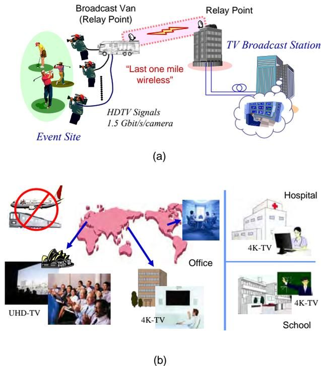
Fig. 6 Application scenes of ultrahigh-speed wireless in access networks.
