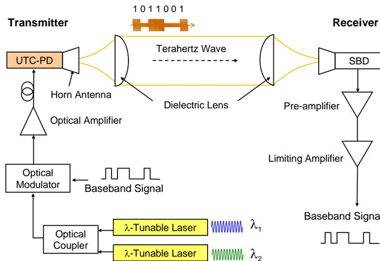
Fig. 11 Block diagram of the wireless link using photonics-based terahertz-wave transmitter.
