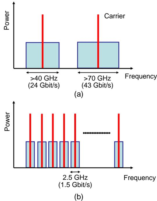
Fig. 9 Possible utilization of 300-500 GHz bands. (a) Ultra-broadband channel. (b) Multiple giga-bit channels.
