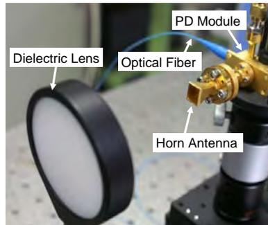
Fig. 12 Photograph of the transmitter with the dielectric lens
