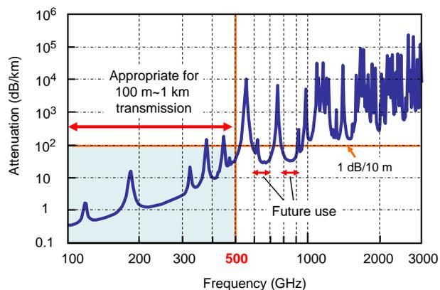
Fig. 8 Atmospheric attenuation of radio waves.
