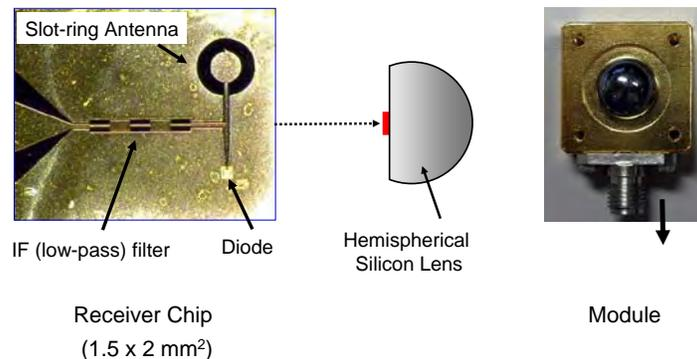
Fig. 15 Photograph of the integrated receiver designed at 250 GHz [11].
