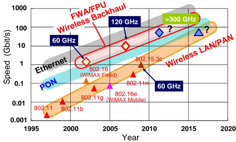
Fig. 3 Trend in wireless communications technologies.
