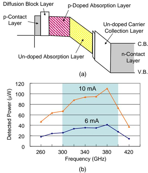
Fig. 10 Band diagram of the photodiode (a), and frequency dependence of output power from the module for photocurrent of 6 mA and 10 mA (b).
