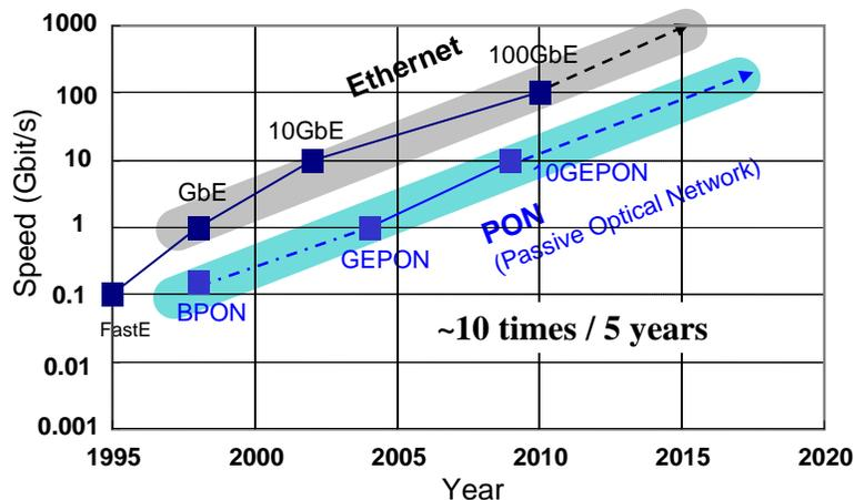
Fig. 2 Trend in wired communications technologies.
