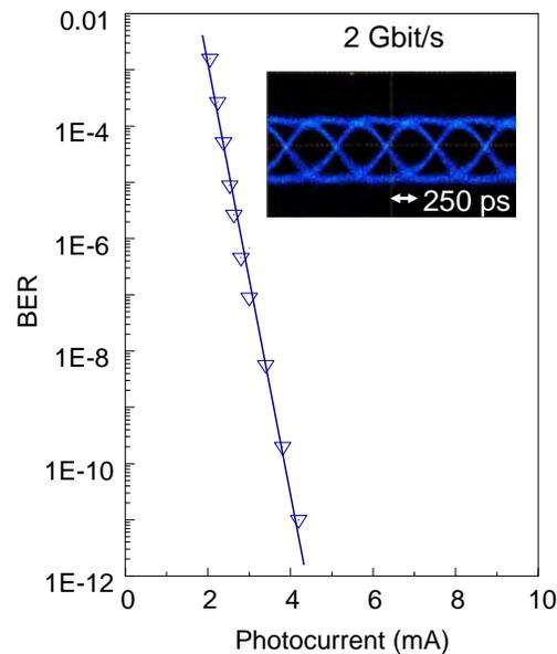
Fig. 13 BER characteristics at 2 Gbit/s with a carrier frequency of 300 GHz. Horizontal axis is a photocurrent of the transmitter
