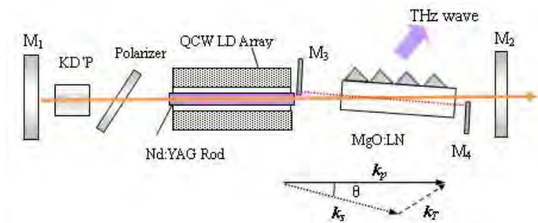
Fig. 1 Schematic diagram of the intracavity THz parametric oscillator
