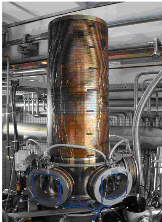
Fig.10 The TED-gyrotron collector with three pairs of TF-coils (the VF-coil is removed)
