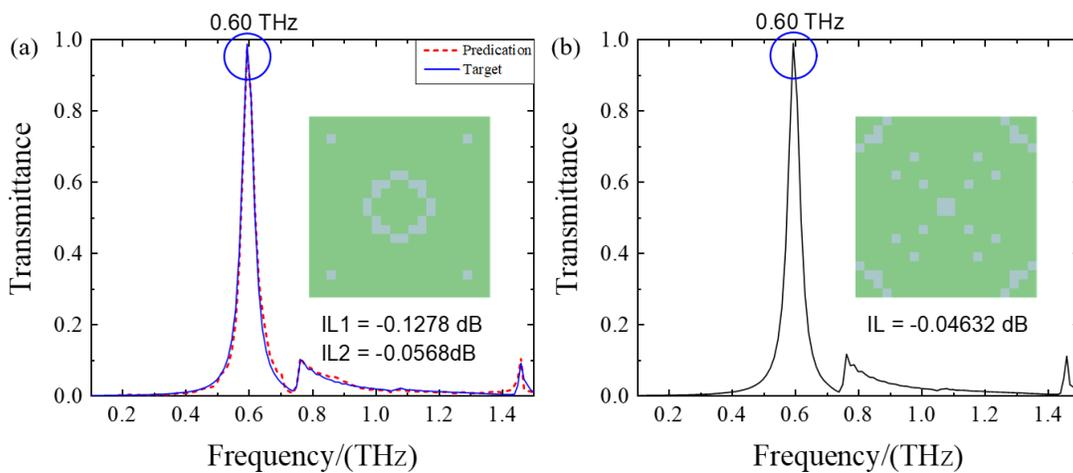
Fig. 8 (a) Convolutional neural network predicted structure and corresponding transmittance; (b) The unit structure and corresponding transmittance curve after BPSO algorithm optimization
