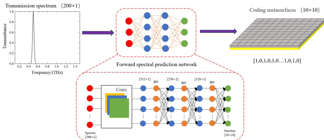
Fig. 3 Reverse prediction network structure diagram
