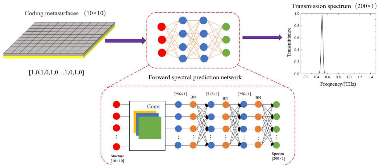
Fig.1 Forward prediction network structure schematic diagram
