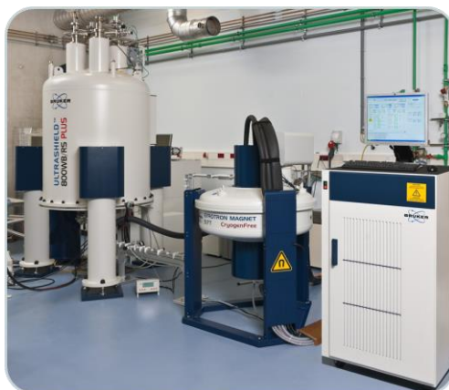
Fig. 10 Photograph of an installed 527GHz/800MHz DNP/NMR spectrometer installed at a Bruker customer site.
