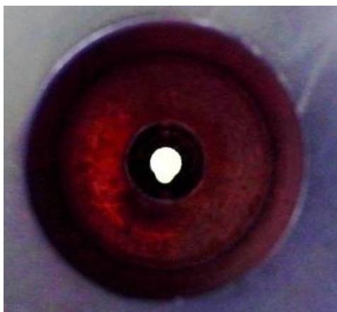
Fig. 1 The photo of an inner groove on the tube wall caused by bombardment of the electrons
