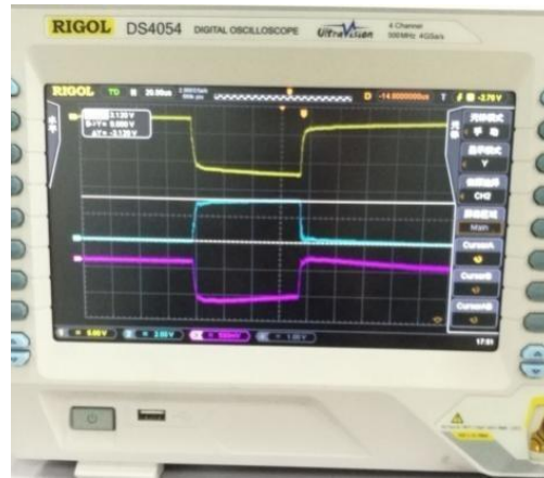
Fig. 10 The measured waveforms of the gyrotron (upper line: operating voltage, middle line: beam current; lower line: output signal)
