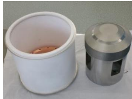
Fig. 3 Photograph of the insulation ceramic and cathode of the single-anode MIG
