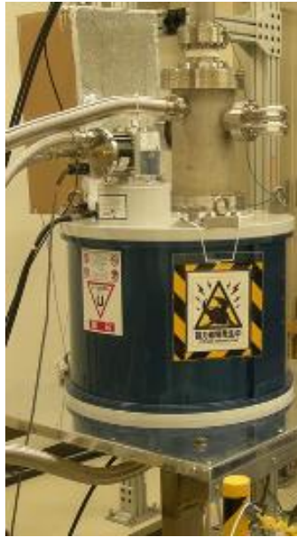
Fig. 2 Photo of the gyrotron FU CW GVI (GO-I) installed at Osaka University, Institute of Protein Research for 700\text{MHz} DNP-NMR spectroscopy.
