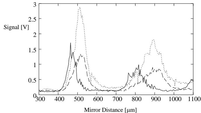
Fig. 8 FP interferograms of the emission at different values of the PMD phase  $\Delta\theta$ : dotted line  $\Delta\theta = 0$  (zero-crossing); dashed line  $\Delta\theta = +9^\circ$ ; solid line  $\Delta\theta = -9^\circ$ . Source [4].
