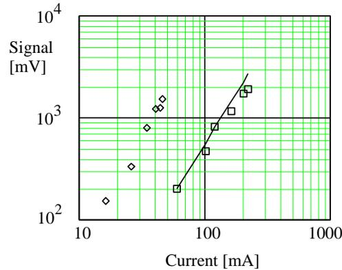
Fig. 7 P4-35 signal as a function of the electron current collected by the upstream (boxes) and downstream (diamonds) targets respectively. The straight line shows the expected quadratic dependence. Source [4].
