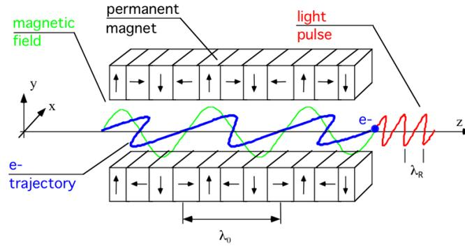
Fig. 1 Geometry of undulator radiation. Source: [http://clio.lcp.u-psud.fr/clio\\_eng/FELrad.html](http://clio.lcp.u-psud.fr/clio_eng/FELrad.html).
