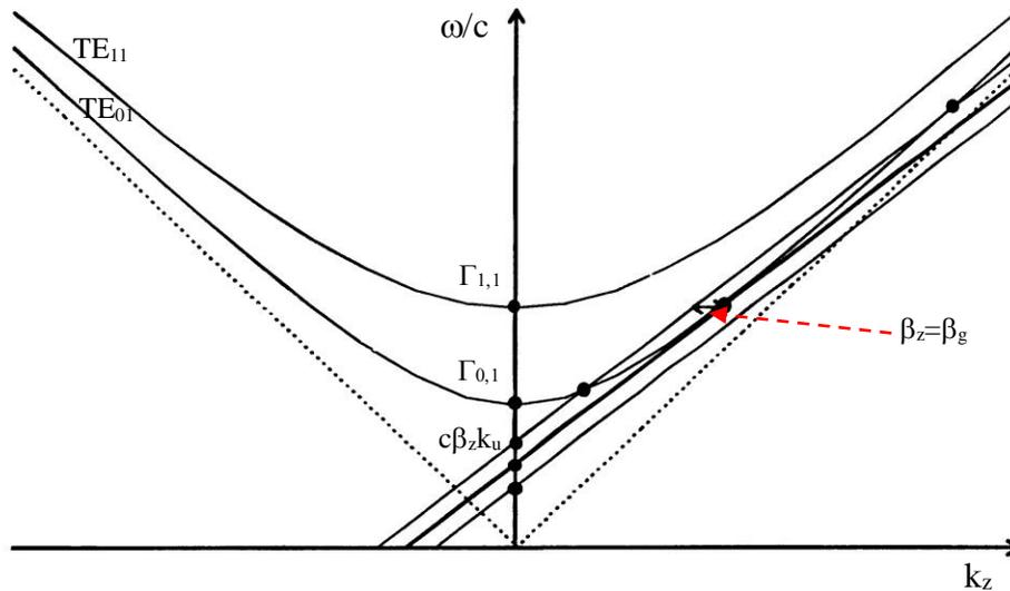
Fig. 2 Graphical representation of the waveguide dispersion relation and the FEL resonance condition (see text for details).
