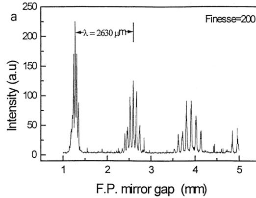
Fig. 5 Fabry-Perot interferogram of the Compact-FEL lasing emission.
