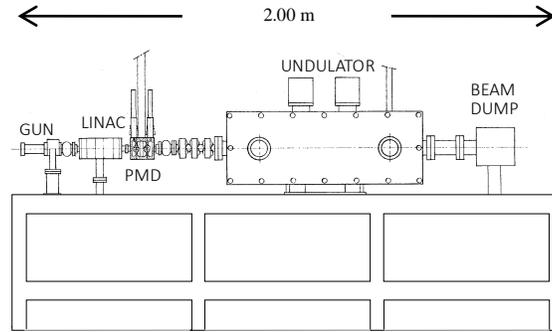
Fig. 6 Lay-out of the FEL-CATS source.
