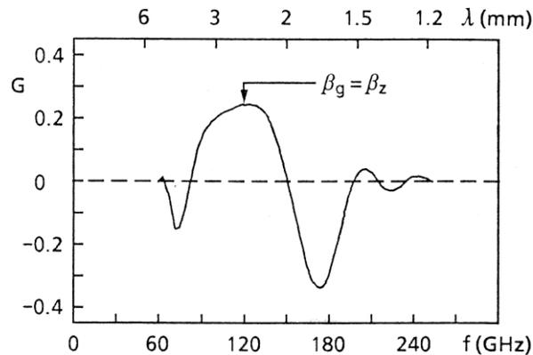
Fig. 4 Calculated gain curve of the Compact-FEL as a function of operation frequency. Source [11]
