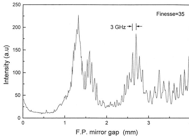
Fig. 3 Fabry-Perot interferogram of the Compact-FEL coherent spontaneous emission.
