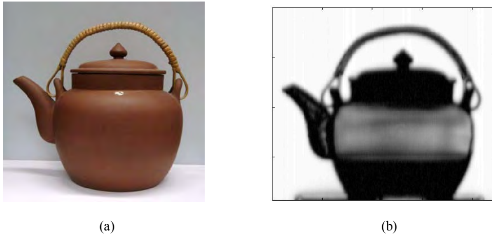
Fig. 7 Photo (a) and THz image (b) of a teapot with some water.
