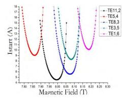
Fig. 4 Starting currents for six modes as a function of magnetic field.
