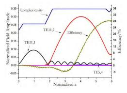
Fig. 5 Field profile and interaction efficiency
