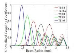
Fig. 3 Coupling coefficients for several modes as a function of R<sub>b</sub>.
