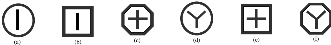
Fig. 2 Several dualband configurations of combined of traditional FSS elements: (a) diople/ring, (b) dipole/square loop, (c) crossed dipole/hexagon loop, (d) three-legged dipole/ring, (e) crossed dipole/square loop and (f) three-legged dipole/hexagon loop.
