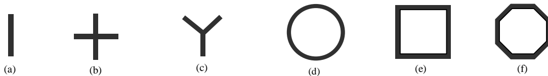
Fig. 1 Basic element structures of the conventional FSS resonator can be divided to type A: (a) dipole, (b) crossed dipole, (c) three-legged dipole, and type B: (d) ring, (e) square loop, and (f) hexagon loop.
