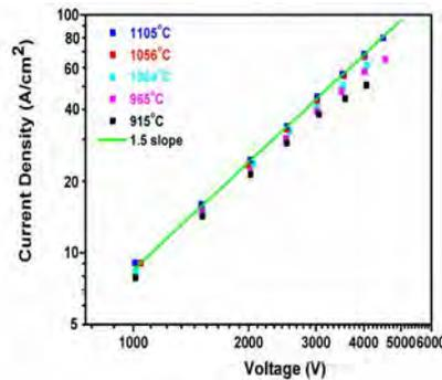
Fig. 9 Emission characteristics of nanocomposite cathode made by using 500-700 nm powder at different cathode temperatures.
