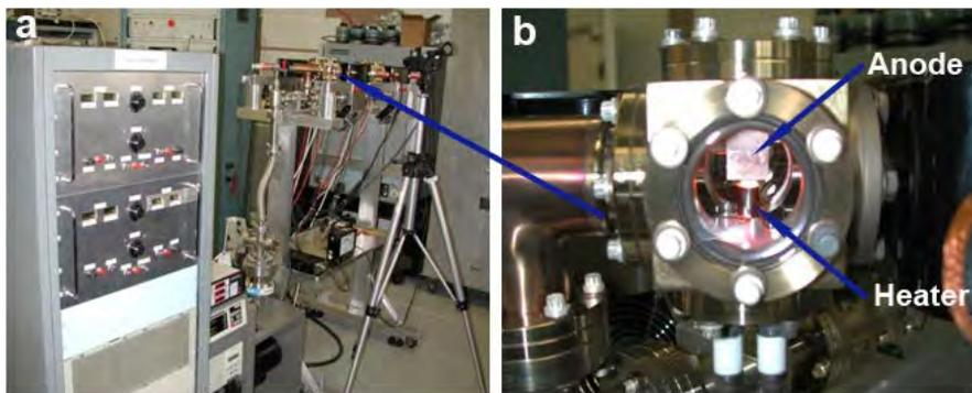
Fig. 5 (a) Cathode testing UHV cube systems with four cubes; (b) One cathode testing cube employing a CSD configuration.
