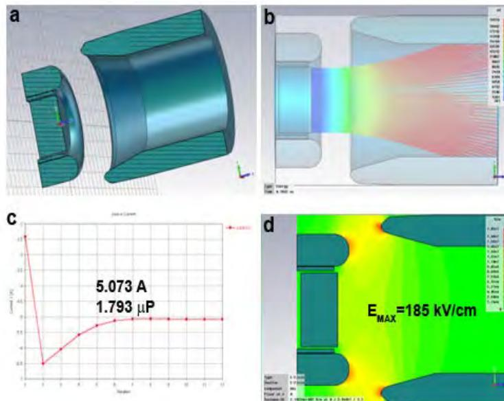
Fig. 7 (a) Electron gun model that includes cathode, focus electrode, and anode/collector; (b) Electron beam trajectory being dissipated in the anode/collector; (c) Extracted current  $5.073\text{ A}$ ; (d) Electric field lines contour plot showing a maximum field of  $\sim 185\text{ kV/cm}$ .
