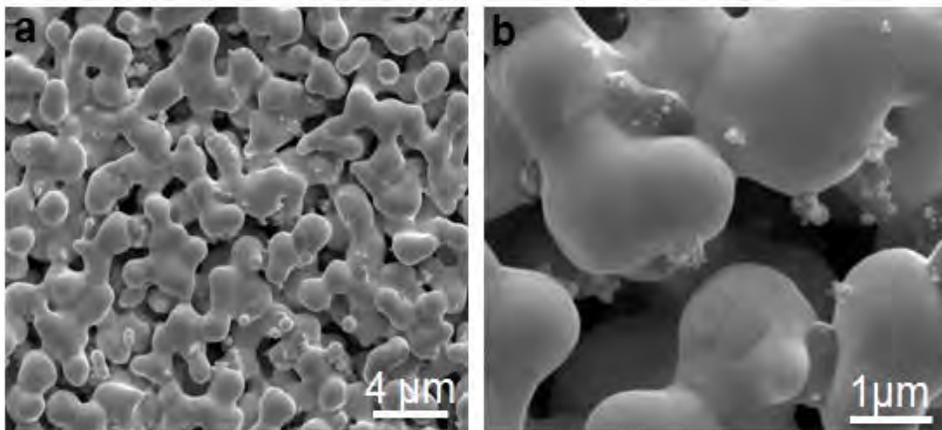
Fig. 2 (a) and (b) SEM images of scandate dispenser cathode pellet made from 1-2  $\mu\text{m}$  powder with different magnifications.
