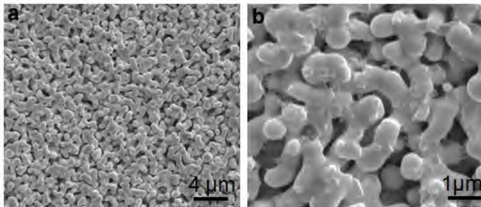
Fig. 1 (a) and (b) SEM images of scandate dispenser cathode pellet made from 500-700 nm powder with different magnifications.
