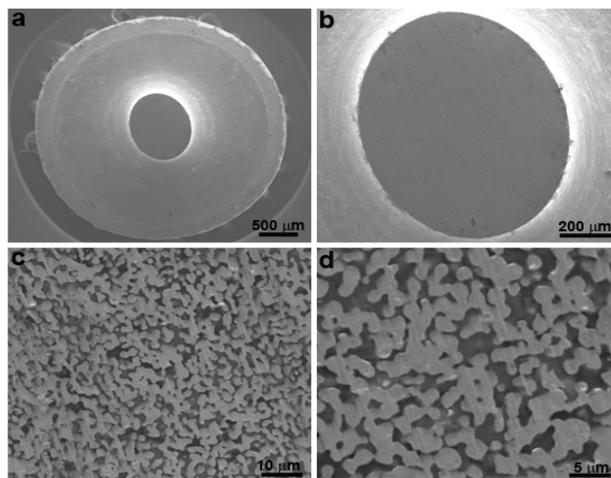
Fig. 4 SEM images of the machined elliptical scandate dispenser cathode made from  $1\text{-}2\text{ }\mu\text{m}$  powder with different magnifications.
