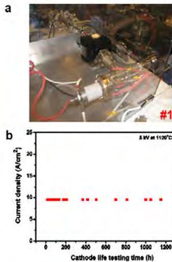
Fig. 10 (a) Cathode life testing vehicle #1 under CW testing; (b) The life testing results of CLTV #1 at  $1120^\circ\text{C}$  and 5 kV.
