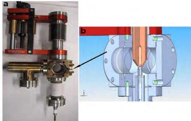
Fig. 6 (a) Modified UHV cube with real gun configuration; (b) schematic drawing of the inner structure of the Modified cube including the collector, focus electrode, cathode and heater etc.
