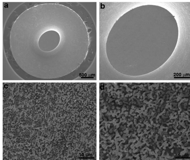
Fig. 3 SEM images of the machined elliptical scandate dispenser cathode made from  $500\text{-}700\text{ nm}$  powder with different magnifications.
