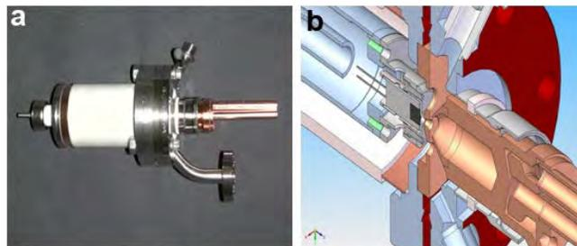
Fig. 8 (a) (b) schematic picture and drawing of cathode life testing vehicle for both pulsed and CW testing.
