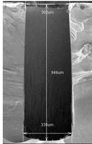
Fig. 22 Cross section SEM view of the serpentine trench fabricated by the first step DRIE, it can be seen that the width is about 302\mu\text{m} on the top and is 335\mu\text{m} at the bottom of the trench, and the depth is 946\mu\text{m} .
