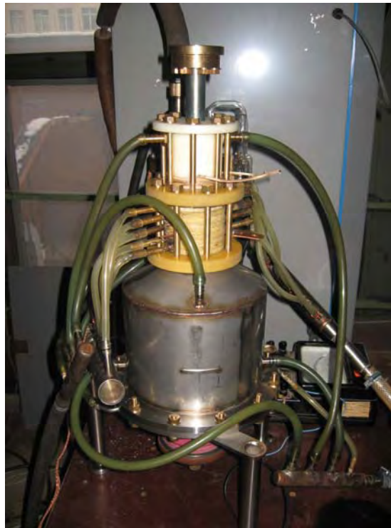
Fig. 6 The general view of MW level gyrotron with operating frequency about 0.3\text{ THz}
